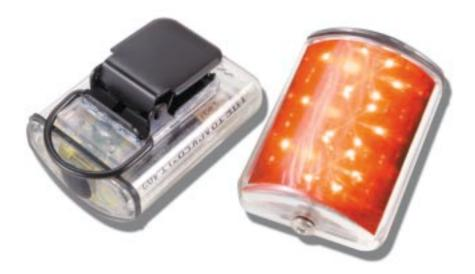
The Lite-Tracker is a flashing visual indicator intended to show the position of personnel working in areas of bad visibility. It is a small lightweight unit fitted with two primary batteries which feed an extremely bright LED light source which, with its blinking flashing effect, penetrates darkness and smoke. The scattering lens fitted enables the Lite-Tracker to spread the light over a wide angle.
